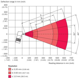
① Diagram applies to focus position of 280 mm
