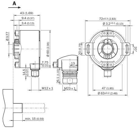
General tolerances according to DIN ISO 2768-mk ① Cable diameter = 5.6 mm +/- 0.2 mm bend radius = 30 mm
