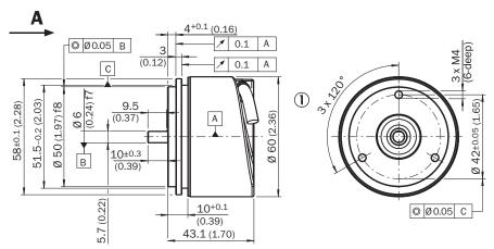
General tolerances according to DIN ISO 2768-mk  $\odot$  Cable diameter = 5.6 mm +/- 0.2 mm bend radius = 30 mm
