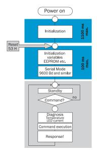
CAUTION: No **RS485 communication** is possible during the phases highlighted in blue Signal diagram for clockwise shaft rotation, looking in direction "A" (see dimensional drawing) 1 period =  $360^{\circ}$ : 16
