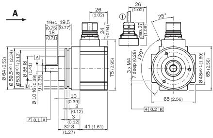
① R = min. bending radius 40 mm
