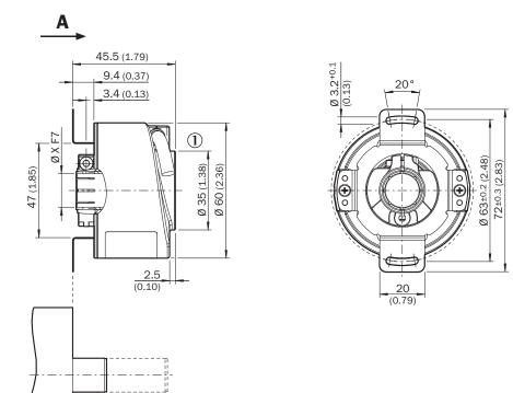
General tolerances according to DIN ISO 2768-mk ① Cable diameter = 5.6 mm +/- 0.2 mm bend radius = 30 mm
