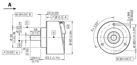
General tolerances according to DIN ISO 2768-mk  $\odot$  Cable diameter = 5.6 mm +/- 0.2 mm bend radius = 30 mm
