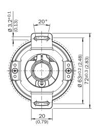
General tolerances according to DIN ISO 2768-mk  $\odot$  Cable diameter = 5.6 mm +/- 0.2 mm bend radius = 30 mm
