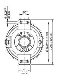
General tolerances according to DIN ISO 2768-mk (1) Cable diameter = 5.6 mm +/- 0.2 mm bend radius = 30 mm
