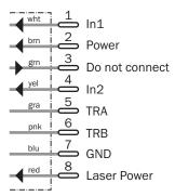
Connection diagram, encoder connection
